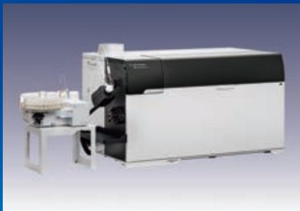
■誘導結合プラズマ質量分析計 (ICP-MS/MS) ■Inductively Coupled Plasma Mass Spectrometer (ICP-MS/MS)
